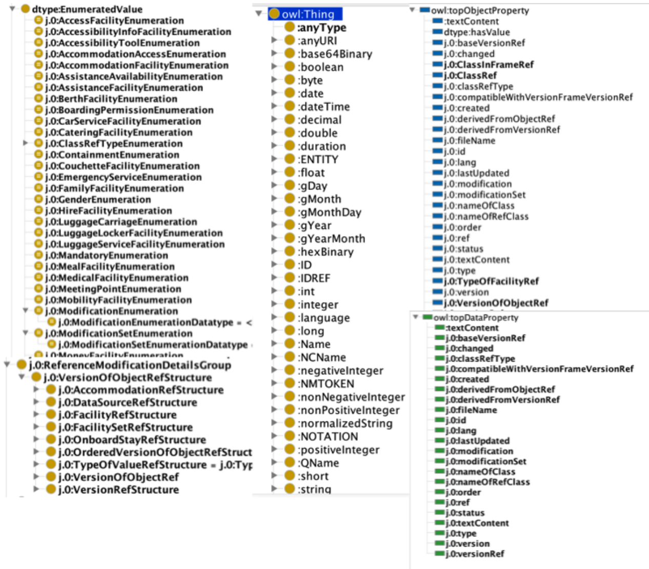
Figure 3. Some classes and properties automatically generated from an XML Schema file from NeTex
